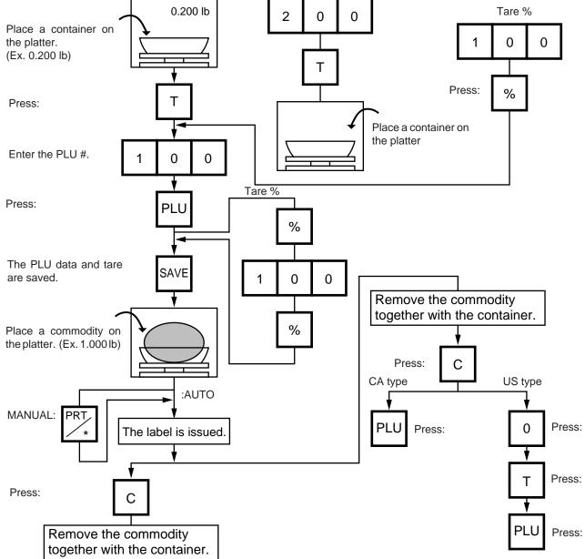
NOTES: 1. Tare subtraction is available up to 2.000 lb. for US type, and up to 1.000kg (2.205lb) for the CA/QR/AU type. When tare subtraction is in operation, however, the scalable range for net weight becomes less by the amount of the tare. (Net weight = Gross weight-Tare)
